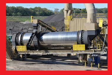
By the innovative flight design, the aggregates curtain is formed immediately after the feeding section, and keeps smoothly moving forward upto the burner chamber, then, flows towards the discharge chute no longer forming aggregates curtain, Dryer support rollers are fixed on the frame with a cerrtain pin, so,the dryer position shall noot be changed, and factory pre-alignment is widely applied for easy adjustment
