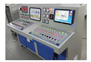
The control is equipped with function keys and numeric keys and does not require special skills for operationDisplay of all process control parameters
